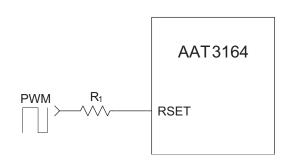
Figure 4: RSET Configuration for PWM Dimming Control.
