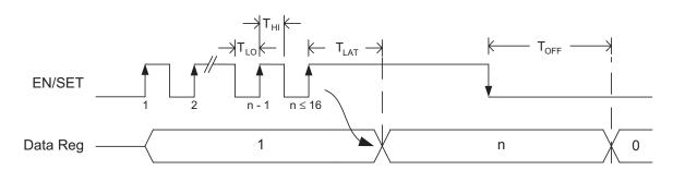
Figure 1: S<sup>2</sup>Cwire Serial Interface Timing Diagram.
