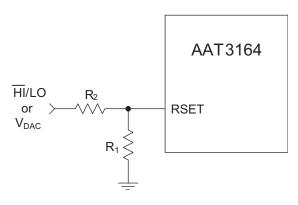
Figure 3: RSET Configuration Using Two Resistors.
