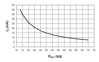
Figure 2: Maximum LED Current vs. R<sub>SET</sub>.
