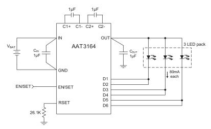
Figure 5: Configuration for a Typical Three-LED Application.
