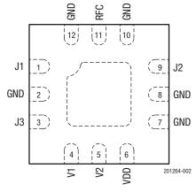
Figure 2. SKY13373-460LF Pinout (Top View)
