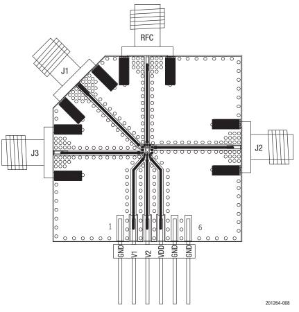
Figure 8. SKY13373-460LF Evaluation Board Assembly Diagram
