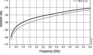
**Figure 5. Typical Isolation vs Frequency** (RFC to J2 Insertion Loss State)
