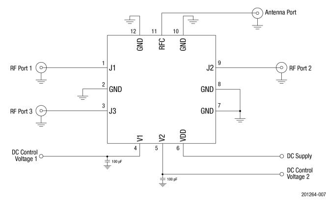
Figure 7. SKY13373-460LF Evaluation Board Schematic
