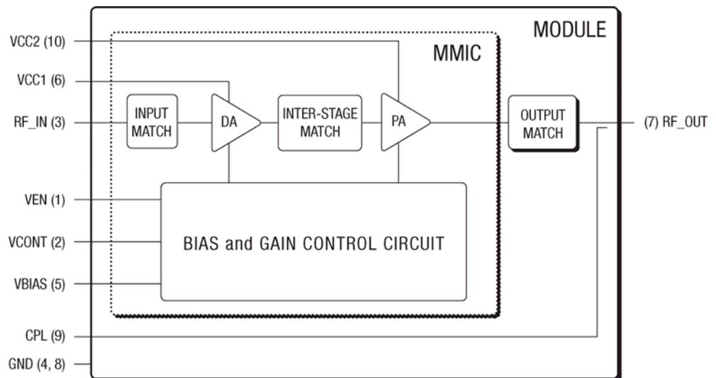
**Figure 1. SKY77446 Functional Block Diagram**
