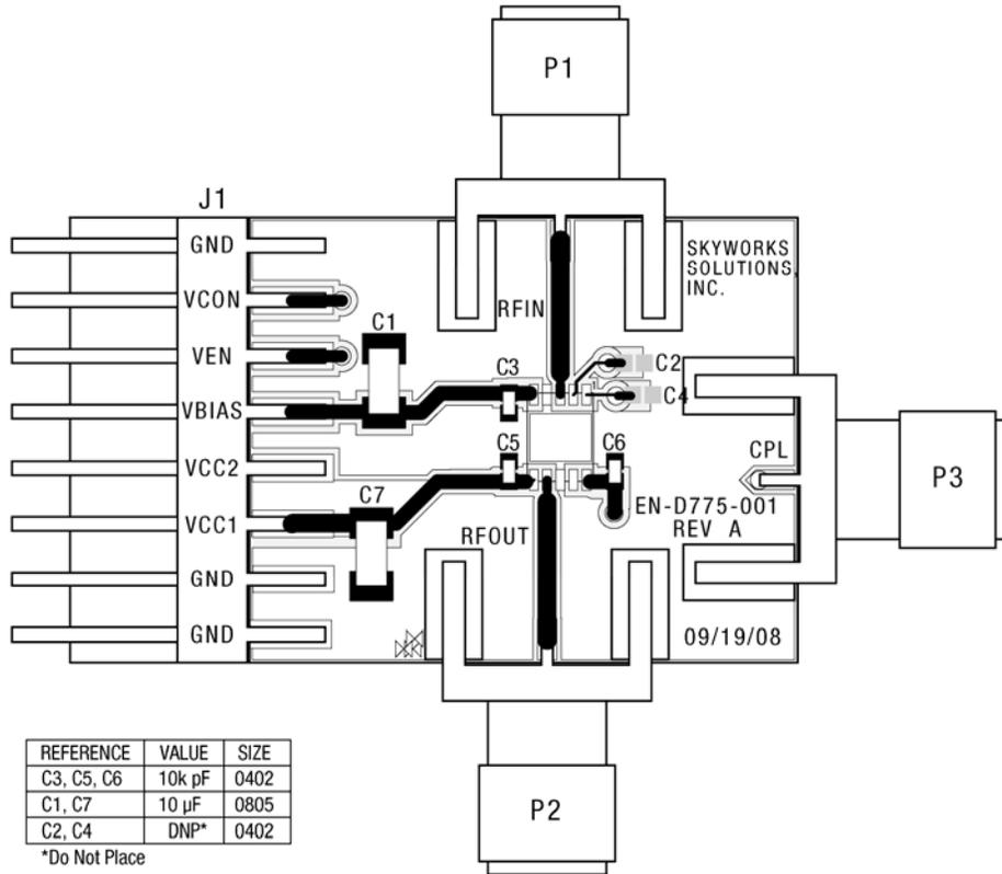
Figure 3. Evaluation Board Assembly Diagram
