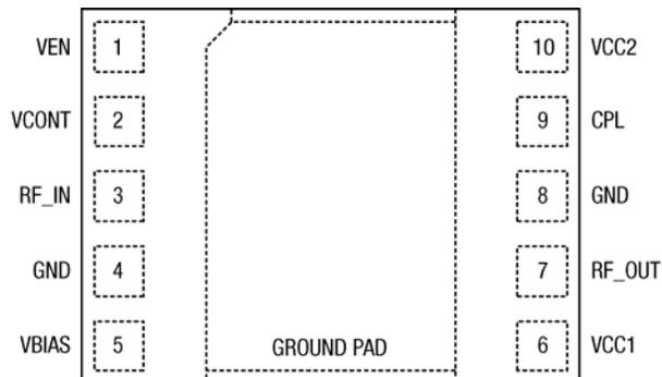
Pad layout as seen from Top View looking through the package. GROUND PAD is package underside.
