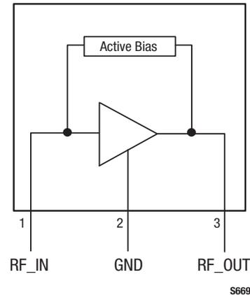
Figure 1. SKY65081-70LF Functional Block Diagram
