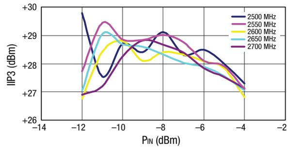
**Figure 8. IIP3 vs Input Power Over Frequency**
