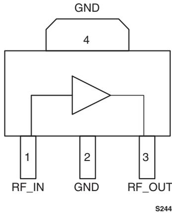
**Figure 2. SKY65081-70LF Pinout (Top View)**
