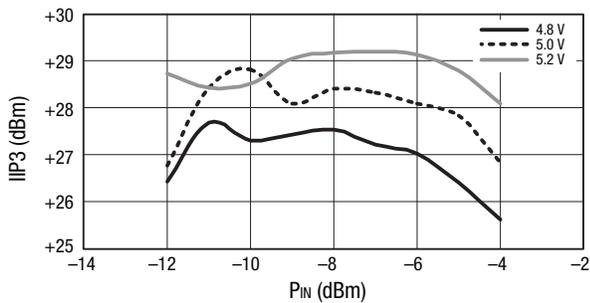
**Figure 9. IIP3 vs Input Power Over Voltage**
