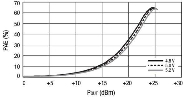
Figure 11. PAE vs Output Power Over Voltage
