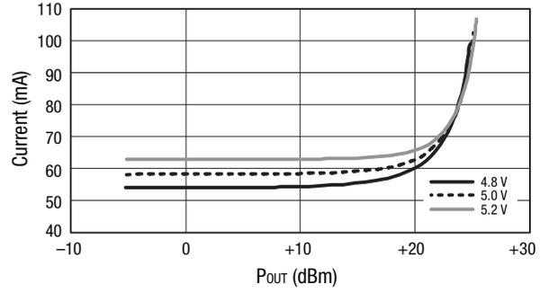
Figure 12. Current vs Output Power Over Voltage
