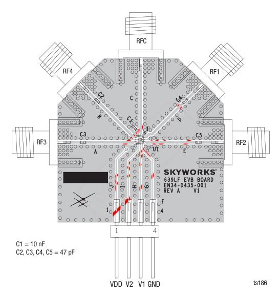
Figure 4. SKY13524-639LF Evaluation Board Assembly Diagram
