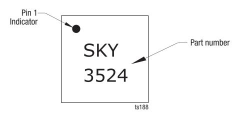
Figure 6. Typical Part Markings (Top View)
