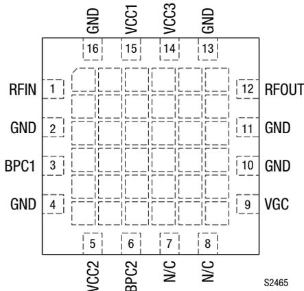
**Figure 2. SKY65372-11 Pinout (Top View)**
