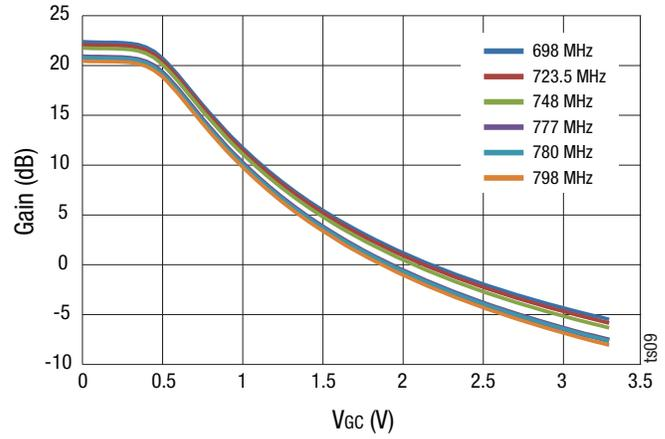
**Figure 8. Low Gain vs V<sub>Gc</sub> over Different Frequency**
