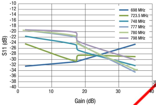
**Figure 3. S11 vs Gain over Different Frequency**
