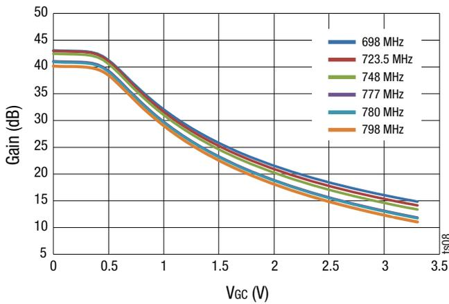
**Figure 7. High Gain vs V<sub>Gc</sub> over Different Frequency**
