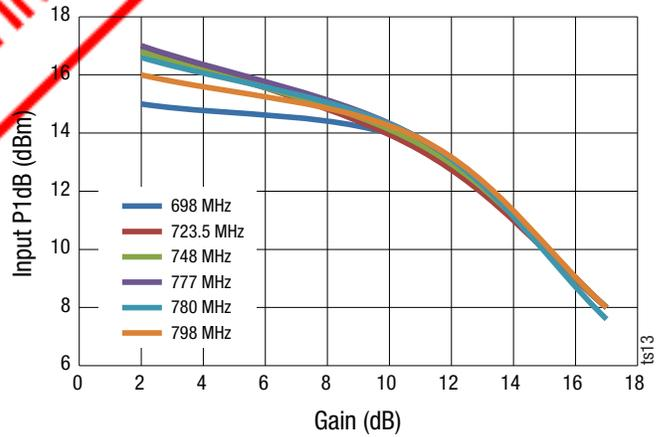
Figure 12. P1dB vs Low Gain Setting over Different Frequency
