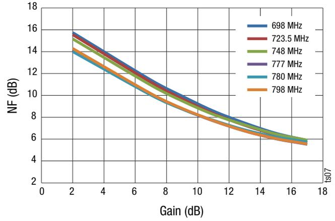
**Figure 6. NF vs Low Gain over Different Frequency**
